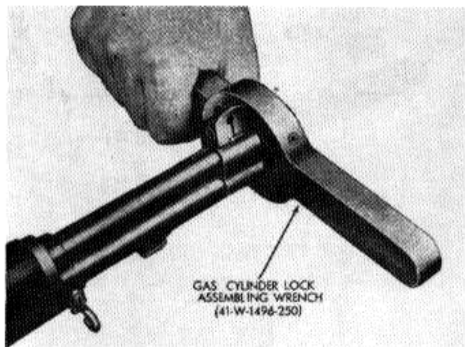
Fig. 115. Removing gas cylinder lock.
